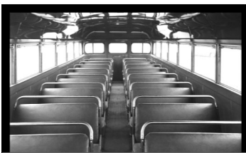
Metal bar seat bracing replaced by high back padded seating.
