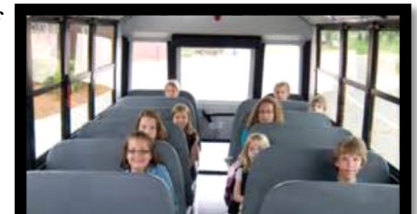
Compartmentalization with impact-absorbing, high-back, padded seats.
