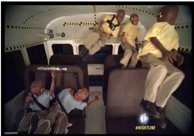
Crash test, left side riders are secured in lap-shoulder seatbelts and on the right, three riders were unbelted.
